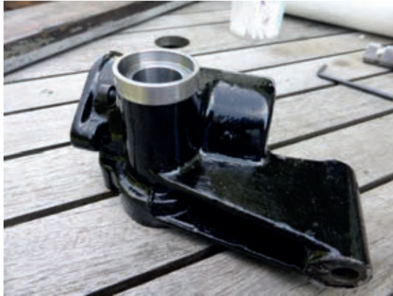
Bush installed (lock-screw not finalized)
