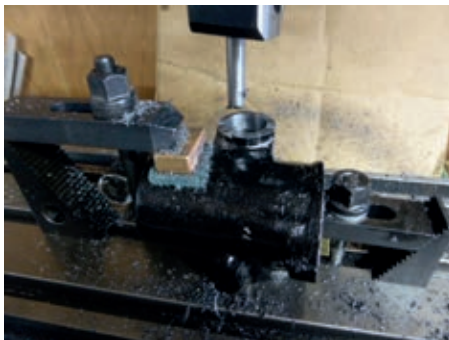
Machining the casing bore to take the bush
