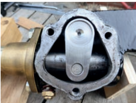
Lever arm at straight ahead position – peg overhangs worm centre-line
